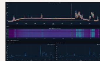
RS205 electric fence badly installed effect on LBA
